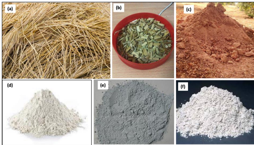
Figure 1. Materials used for brick fabrication (a-b)Rice straw (c) Laterite Soil (d) Lime (e) Portland Cement (f) GGBS
