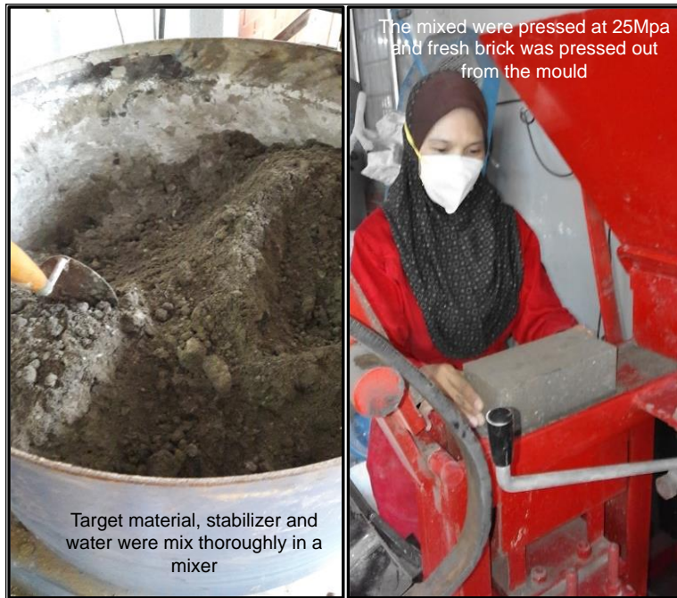
Figure 2. Materials were thoroughly mixed and pressed. Fabrication of LSP Bricks
